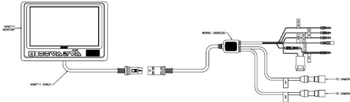
Install the **AOM713** monitor panel to existing mount and connect to existing harness connection.
