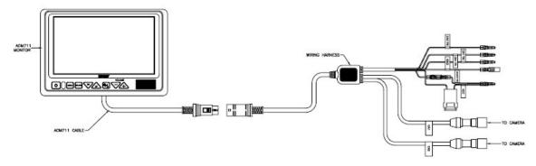
Install the **AOM713** monitor panel to existing mount and connect to existing harness connection.
